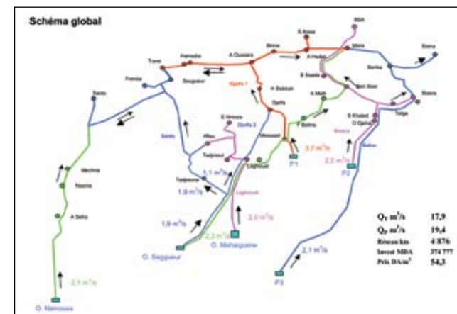
Map showing transfer of water between regions in Algeria. Water prices are controlled across the country to ensure affordability.
