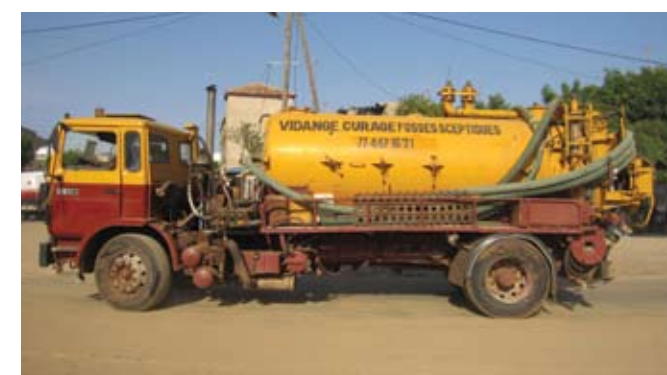
Tanker for collecting waste from septic tanks in a high-density settlement, in Rifisque, Dakar, Senegal, November 2011.
